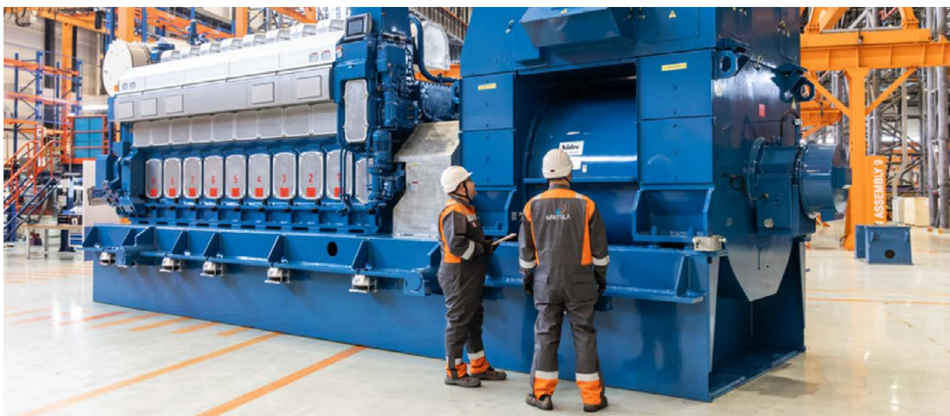
Figure 1: Wartsila's RICE technology is a large internal combustion engine that can be deployed modularly to fit the needs of any high-renewables power system.
